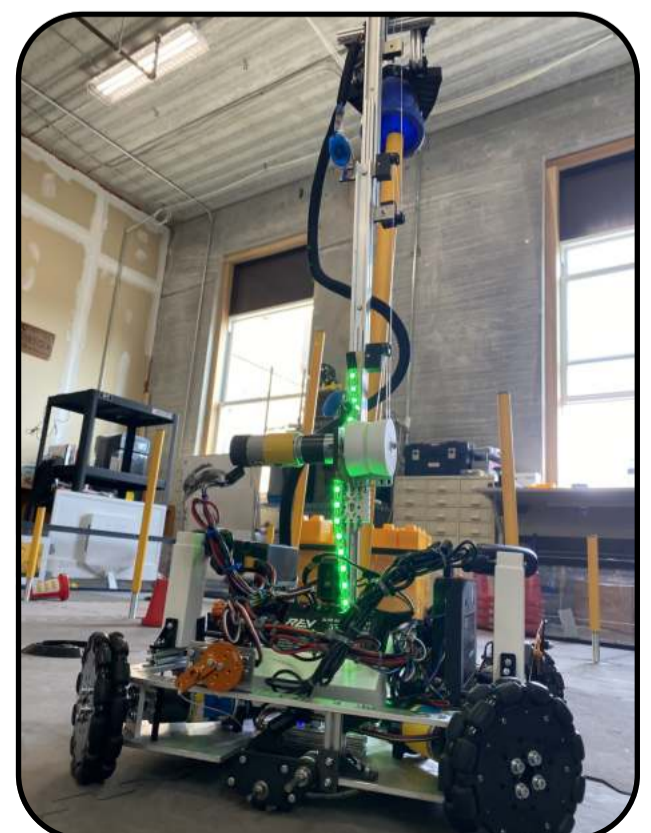
Right: Here, our LEDs are turning green to signal that we are in line with the pole, utilizing our webcam stereo processing algorithm (detailed on the next page).
